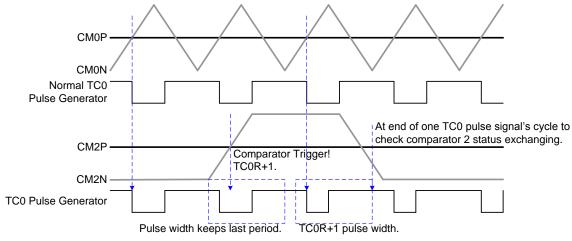
Step 2: If comparator output status doesn't exchange, TC0R + 1 at the end of one TC0 pulse signal's cycle and outputs the new pulse until comparator 2 output status exchanges.
