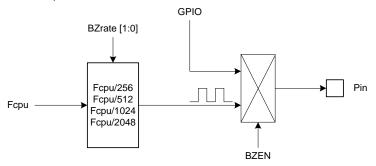
The buzzer frequency is divided from Fcpu (instruction cycle) controlled by BZrate bits, and Fcpu decides the buzzer frequency. The selection table is as following.
