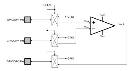
The micro-controller builds in one OP AMP which is Rail-to-Rail structure. That means the input/output voltage is real from Vdd~Vss. The Rail-to-Rail OP AMP pins are shared with GPIO controlled by OPEN bit. When OPEN=0, OP AMP pins are GPIO mode. When OPEN=1, GPIO pins switch to OP AMP and isolate GPIO path. OP pins selection table is as following.
