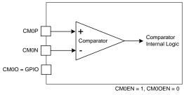
Note: The comparator enable condition is fixed CM0EN=1, or the comparator pins are GPIO mode and comparator is disabled.
