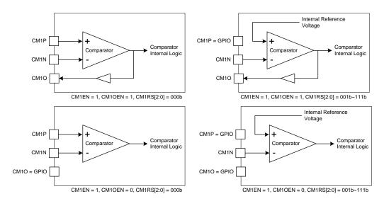
Note: The comparator enable condition is fixed CM1EN=1, or the comparator pins are GPIO mode and comparator is disabled.
