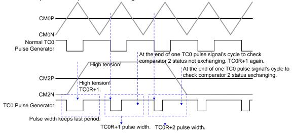
Note: If TC0R is increased to 0xFF, TC0R will keep 0xFF and not increase again, even the comparator output status never occurs exchanging.
