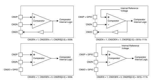
Note: The comparator enable condition is fixed CM2EN=1, or the comparator pins are GPIO mode and comparator is disabled.
