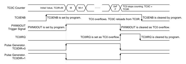
If the trigger is comparator 0 output edge (rising edge and falling edge controlled by comparator control register's CM0G bit), pulse starts to output as trigger edge condition occurrence. When TC0 overflows, pulse output pin returns to idle status.
