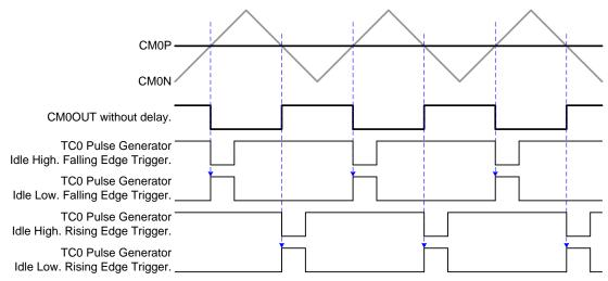
TC0 pulse generator output signal without delay.
