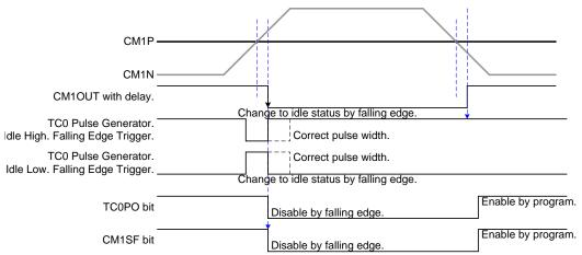
Stop TC0 pulse output @falling edge trigger, with delay.
