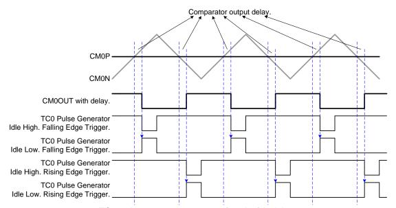
TC0 pulse generator output signal with delay.
